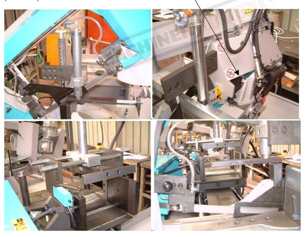
Minimal lubrication system - This device, applied to the saw, allows to eliminate almost completely the traditional coolant system, keeps the material much cleaner and avoids to waste cutting oil and water. It works only during the cut, it is depending from air supply.
