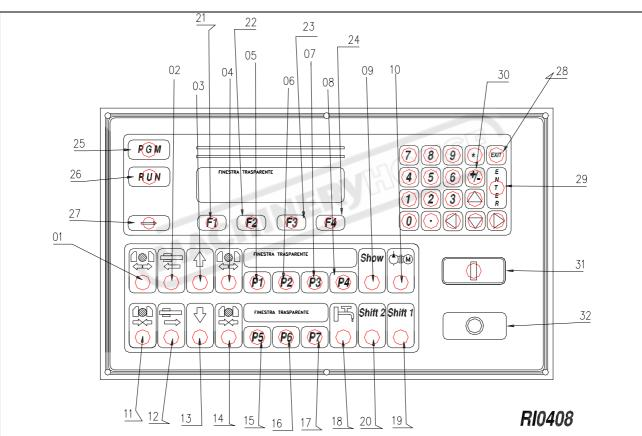
15.2 - KEYBOARD / Description of the buttons and their use - drawing RI0408 All the actions performed by the bandsaw can be programmed by means of the keyboard, including the positioning of the cutting unit:
