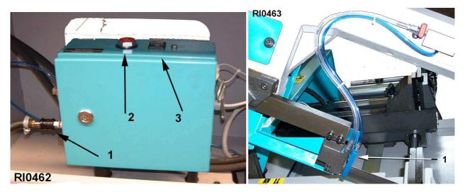
Voltage transformer - place it between the electric supply of the premises and the electric supply of the machine. It allows to work with a different voltage than the standard one (that is 400V / 50 Hz). Available voltages: 230V, 460V, 500V, 575V.
