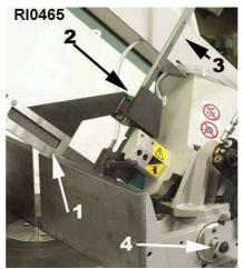
The movement of the sawframe is shown by four symbols:
