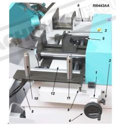
The unloading table - RIGHT SIDE - can be connected directly to the unloading slide thanks to the two lateral holes -14/RI0464.
